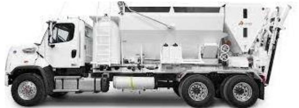
A Volumetric Concrete Truck
